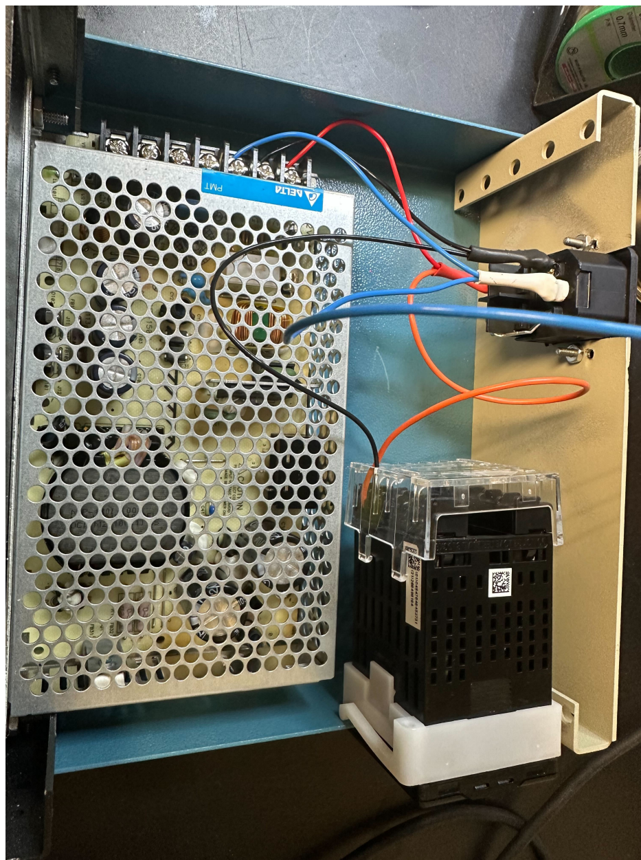
Figure B.13: View of the temperature controller installed inside the box. Holes were drilled to allow a screw to be used to fasten the controller to the bottom portion of the box. Another hole is used for the top part of the box.
