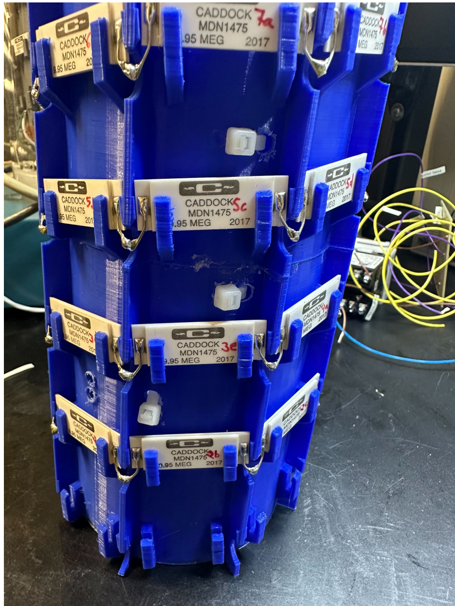
Figure B.19: HV resistors installed in a spiral pattern around the 3d-printed column. Note the zipties, which are used to hold the thermocouple in place. Also note that the 3d-printed columns are glued together.
