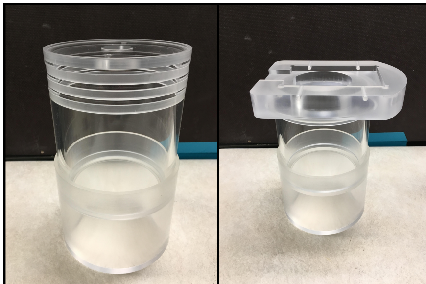
Figure 6.13: custom-designed gamma-source holder for the LLNL HPGe detector.
